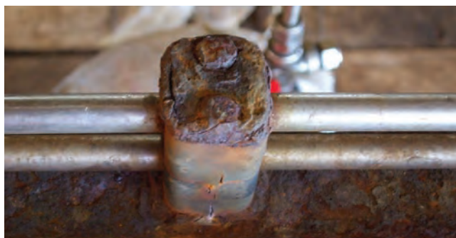
Crevice corrosion between the tube/tube trap interface.
