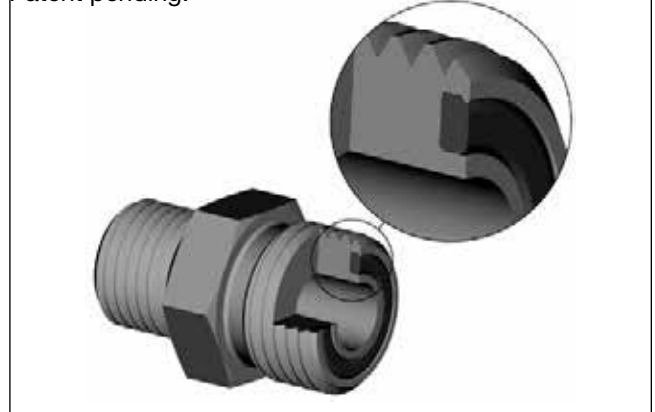
Fig 2 – Captive O-ring Groove (CORG) cutaway
