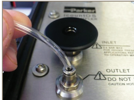
Attach OUTLET (Ø 4mm) hose
