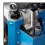
Return stroke limiter. 280.7
