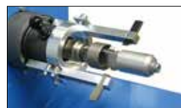
Simultaneous internal and external skiving. (USM 100)
