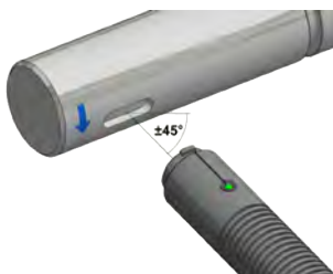
Rotating shaft: Contactless speed measurement.
