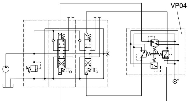
Circuit diagram showing two-section VP04 with one coordinate lever (joystick) controlling one hydraulic directional valve with two spool sections.
