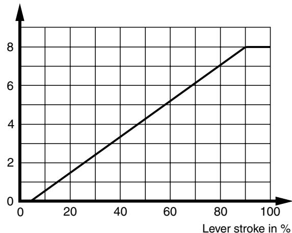
Diagram showing control-pressure characteristic of the VP04-valve. Valid for 8 - 10 bar supply pressure. If lower the curve will level out at obtained supply pressure.
