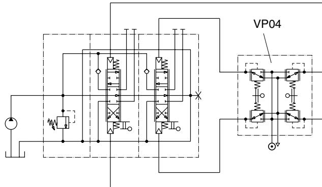
Circuit diagram showing two-section VP04 with two linear levers controlling one hydraulic directional valve with two spool sections.
