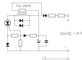
These electrical parts need an external fuse of I = 100 mA
