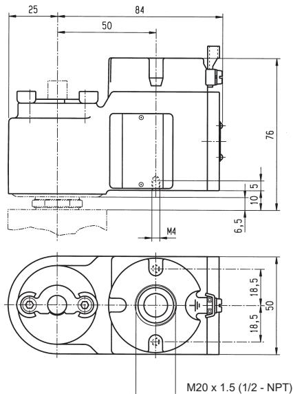
The plunger tube is welded to the stainless steel plate and is thus integrated to the housing which is screwed on the valve body.
