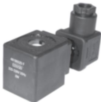
These coils can be mounted with the majority of the Lucifer solenoid valves. This is an encapsulated assembly comprising a coil, integral magnetic iron path and snap-on plug connection. The synthetic material encapsulation provides an effective compact housing, offering full protection against dust, oil, water, etc. Ease of mounting in confined space - offers shock and corrosion protection - simplifies conversion of existing equipment to other requirements, etc.
