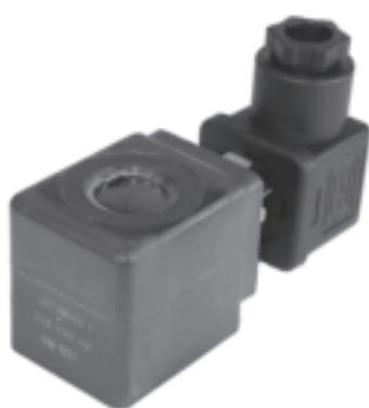
This coil is compatible only with the Offshore and CPR\* types of Lucifer solenoid valves. This is an encapsulated assembly comprising a coil, integral magnetic iron path and snap-on plug connection. The synthetic material encapsulation provides an effective compact housing, offering full protection against dust, oil, water, etc. Ease of mounting in confined space - offers shock and corrosion protection - simplifies conversion of existing equipment to other requirements, etc.
