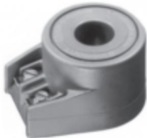
These coils can be mounted with the majority of the Lucifer solenoid valves. They can be mounted with all Lucifer metal housings. The coil winding is completely encapsulated in synthetic material. Easy mounting in confined spaces. Electrical connection with screw terminals for wire up to 1.5 mm".
