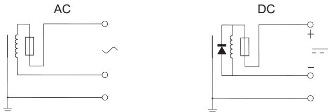
It is necessary to use a safety fuse with a nominal current corresponding to the coil current (max. 3 x nominal according to IEC 60127 and IEC 60269) against short-circuits.
