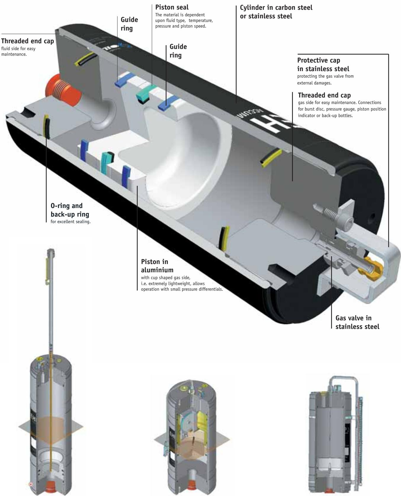
**Piston position indicator.** The piston position indicator is an additional function to the main function of the accumulator, indicating the position of the piston inside the accumulator, thereby ensuring a perfect accumulator operation. The piston position indicator is available with a visual indicator or with electrical monitoring providing 4-20 mA output signal, providing stand-by power during power failure.
