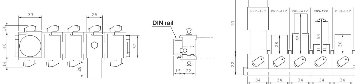
**Relays mounted on 4-port modular sub-bases**
