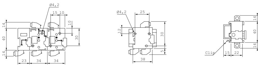
**Relays mounted on 3-port modular sub-bases**
