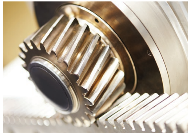
Rack and pinion's drive trains can be ideal for extremely long travel lengths. Rack and pinions typically do not offer much in the way of precision.
