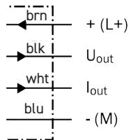
PUR 0.3 meter length with M8 male connector knurled nut, 4-pin
