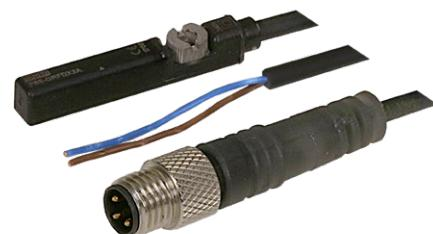
positions. To easy installation there are several cable lengths available with either M8 connector or flying lead. The electronic sensors are "Solid State", i.e. they have no moving parts. They are provided with short-circuit protection and transient protection as standard. The built-in electronics make the sensors suitable for applications with high on and off switching frequency where long service life is required.
