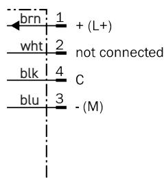
PUR 0.3 meter length with M12 male connector knurled nut, 4-pin
